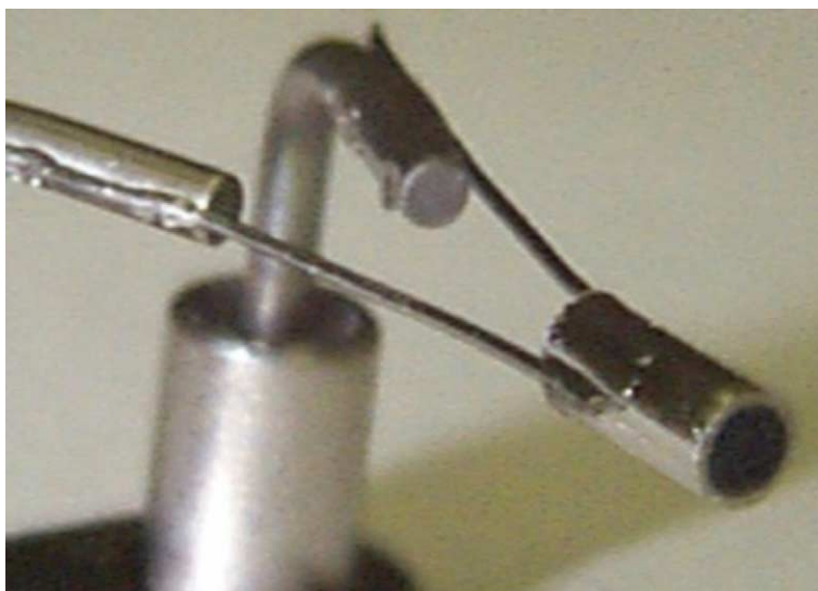
Fig. 3. Re powder/BaSO 4 /metal tube emitters (emitter #42, 1.32 mm o.d.).
