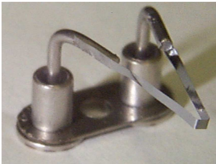
Fig. 2. Re ribbon filament emitters (1 mm wide). Emission is from the square end face.
